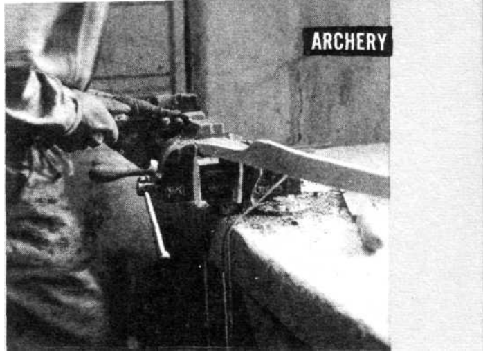
After taking laminated bow from clamps, excess glue must then be removed from handle and limbs.
