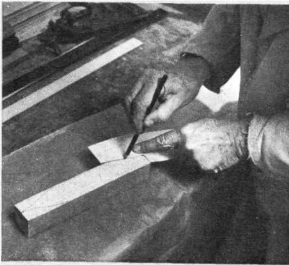
If French curves are unavailable then cut your own patterns in reverse and use them for marking.
